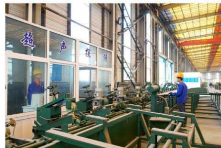
钢管超声探伤检测 UT(Ultrasonic Inspection)
