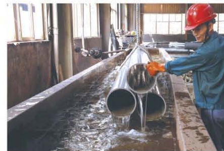
钢管水压检验Hydraulic Test
