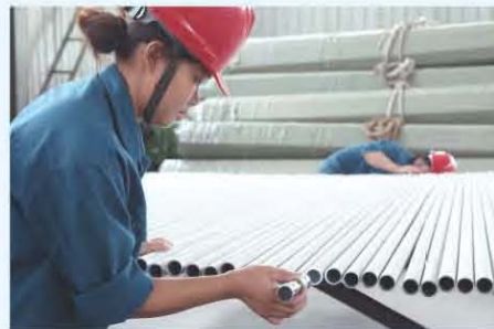
钢管内壁检查 Inside Surface Checking
