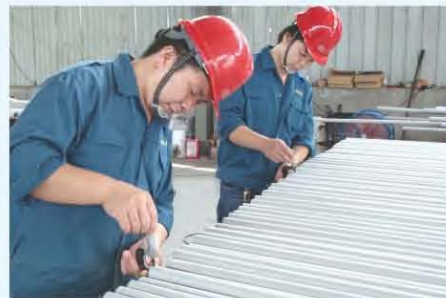
钢管尺寸检验 Thickness Checking
